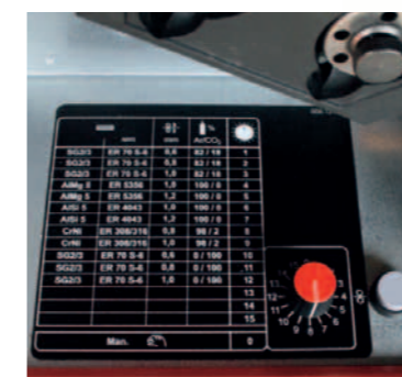
Synergic pre-selection in the BasicPlus and ControlPro models
